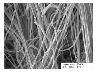
Figure 2. SEM image showing fiber morphology and porosity.
