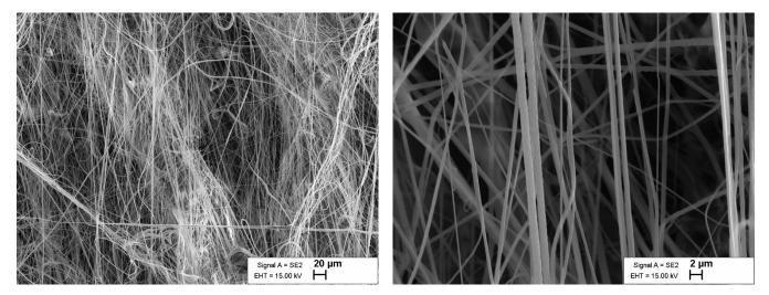
Figure 2. SEM image showing fiber morphology and porosity.
