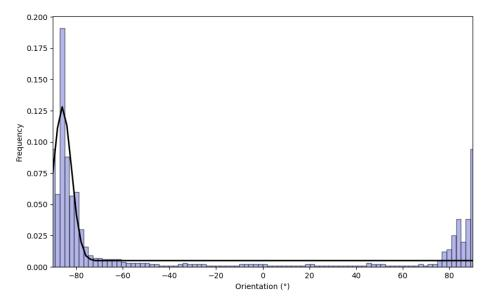
Figure 4. Histogram showing the fiber alignment of a PLLA Aligned scaffold. The exact degree fiber orientation will vary batchto-batch.
