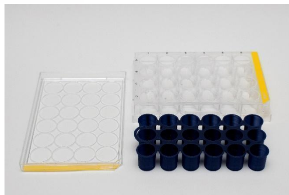
Figure 9. Unpacking Gelacell™ well plate and removing the blue tops.
