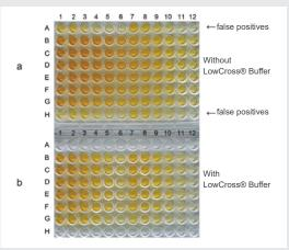
Prevention of false-positive binding in an ELISA against guinea-pig IgG. With the standard assay buffer (a), false positives in the specificity control (row A) and in the blank values (row H) spoiled the interpretations and evaluation. The use of LowCross-Buffer® (b) prevented all false-positive signals.
