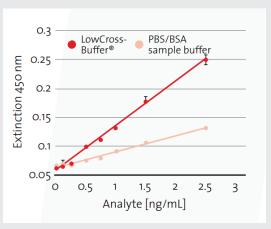
Elimination of a matrix effect. Matrix effect in an assay for detection of CRP (creactive protein) in rabbit blood plasma. Matrix proteins in plasma mask the analyte CRP. LowCross-Buffer® demasks the analyte and improves sensitivity and detection limit by a factor of 3.
