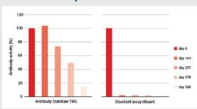
Stress test. Shelf life of an antibody is measured as binding in an ELISA after storage under temperature stress at 45°C. The tests were performed with an antibody concentration of 400ng/mL. After 251 days of incubation with Antibody Stabilizer, the antibody retained around 73% binding activity.
