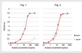
Stress test. Calibration curves of an ELISA, blocked with BSA (fig. 1) or blocked with BSA and stabilized with Liquid Plate Sealer® (fig. 2). Calibration curves at the starting day are identical. After 84 days at 37°C, no remaining binding activity of the capture antibodies is detectable in the unstabilized plate, but the stabilized plate does not show a significant decrease in sensitivity.
