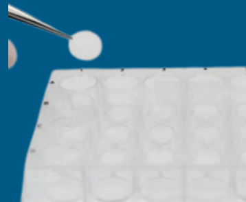
Well Plate with Scaffold
