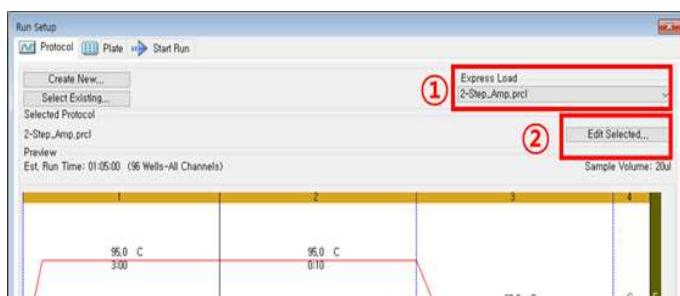
③ In the Protocol Editor window, configure the PCR cycling conditions (see “PCR Amplification”, page 12). Use the <Insert Step> button at the lower left to add cycling steps, and set the temperature and time parameters in the fields located in the center of the window. After confirming all entries, click <Save>, followed by <OK>, to store the PCR protocol.
