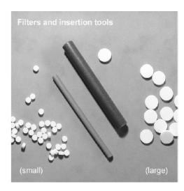
Small and large filters with different diameters (10  $\mu$ m, 35  $\mu$ m and 90  $\mu$ m) are separately available, so you can use the filter of your choice.
