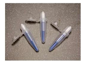
The Isohelix **Spin+Collect** firmly grips the swab or other material whilst exposing maximal surface area for the first step of elution or lysis of the sample. A 1.5ml microfuge tube is then fitted as a cap and inverted for centrifugation and final release of any sample trapped in the matrix.
