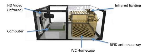
Figure 1: Schematic of the Home Cage Analysis System.
