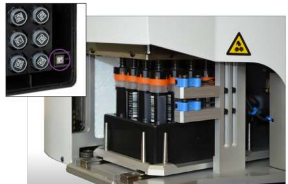
New design swab cap suitable for automated decapping and liquid handling systems
