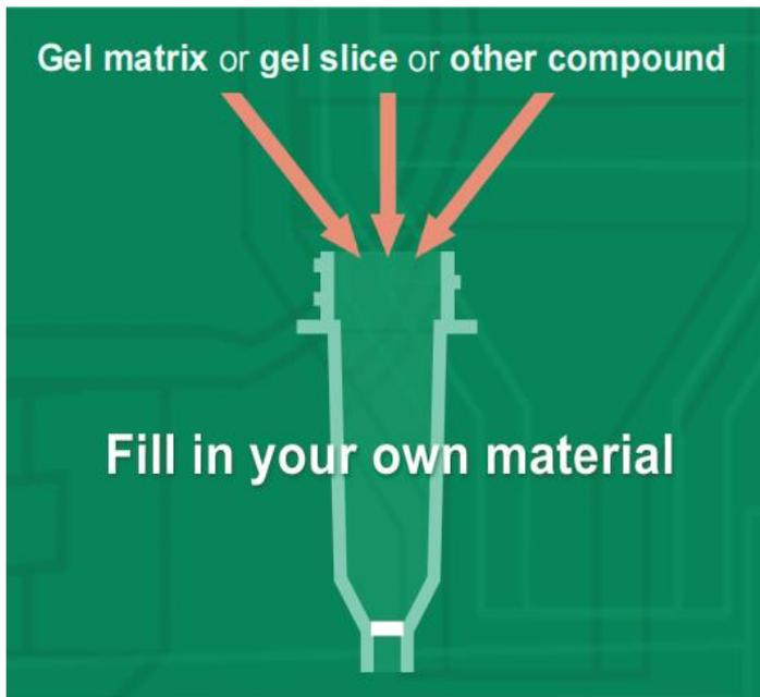
The MobiSpin Column "F" is designed for a wide variety of applications for nucleic acid and protein extraction and purification. When choosing the MobiSpin Column "F" for a particular application, a suitable resin must be selected and filled into the mini-column. For an appropriate resin selection, impurity versus sample size and the anticipated yield must be considered.
