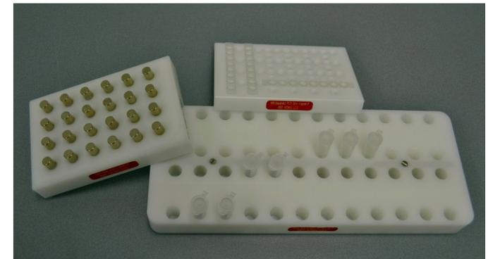
Fig 4: POM versions of the manual separators
