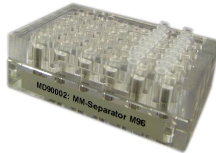
Fig. 4: MM-Separator PCR strip adapter.
