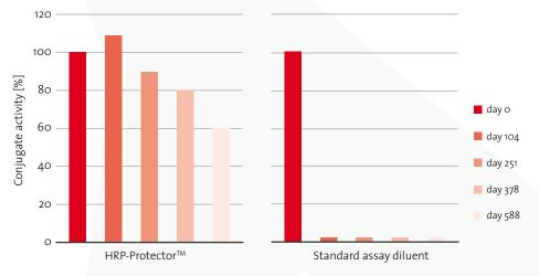
Shelf life of an HRP-labeled antibody is measured as signal (= antibody binding + enzymatic activity) in an ELISA after storage under heat stress at  $45^{\circ}$ C. The concentration of the stored antibody is  $400\,\text{ng}$ /mL.
